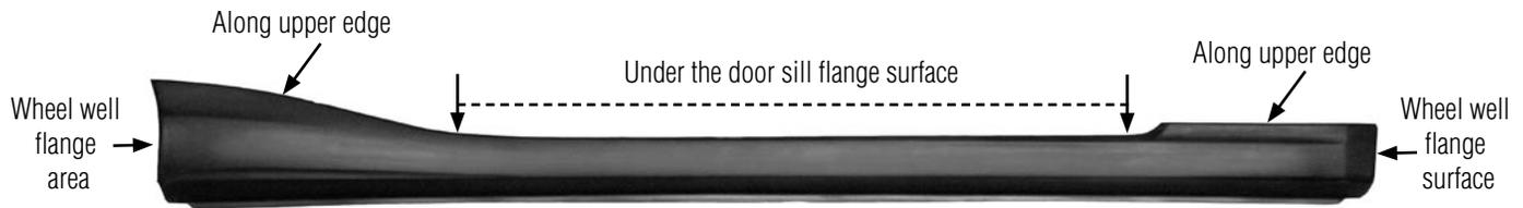
7. Use acetone to clean the bonding areas (see noted areas of the photo below). NOTE: Acetone will attack the paint if given time - move quickly with the rag!
